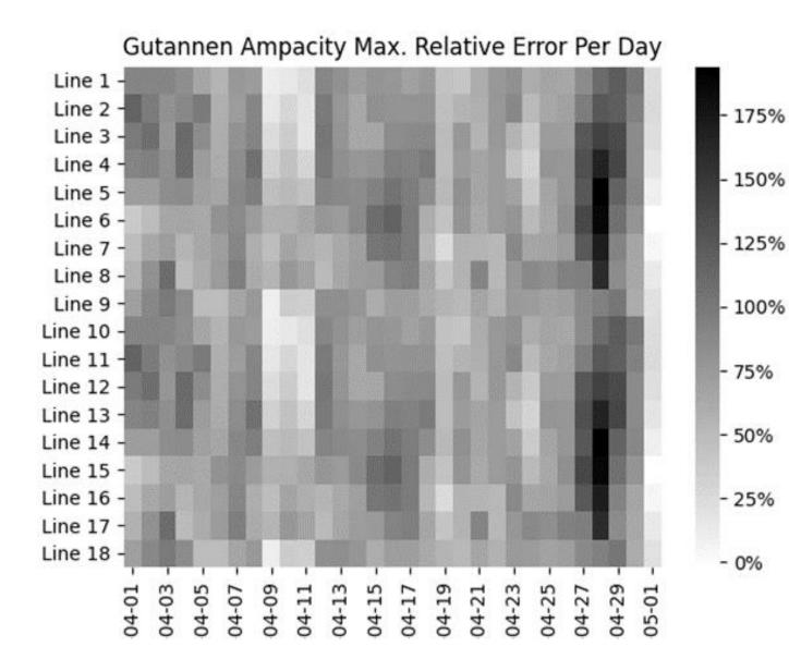
Effect of Wind Direction Prediction **Horizontal Axis** Date (April 2021 – May 2021) **Vertical Axis** Imaginary OHL, each with a 20° offset Greyscale **Error Rate Conclusion:** The maximum Error is more than 175% (on 04-28)
