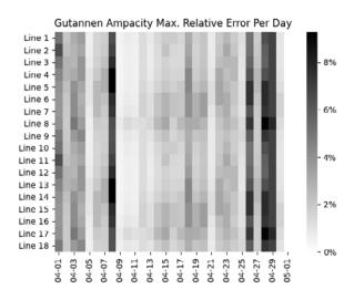
**Wind Direction** Gutannen Ampacity Max. Relative Error Per Day Line 1 Line 2 40% Line 3 Line 4 Line 5 Line 6 30% Line 7 Line 8 Line 9 20% Line 10 Line 11 Line 12 10% Line 14 Line 15 Line 1€ 0% Line 18
