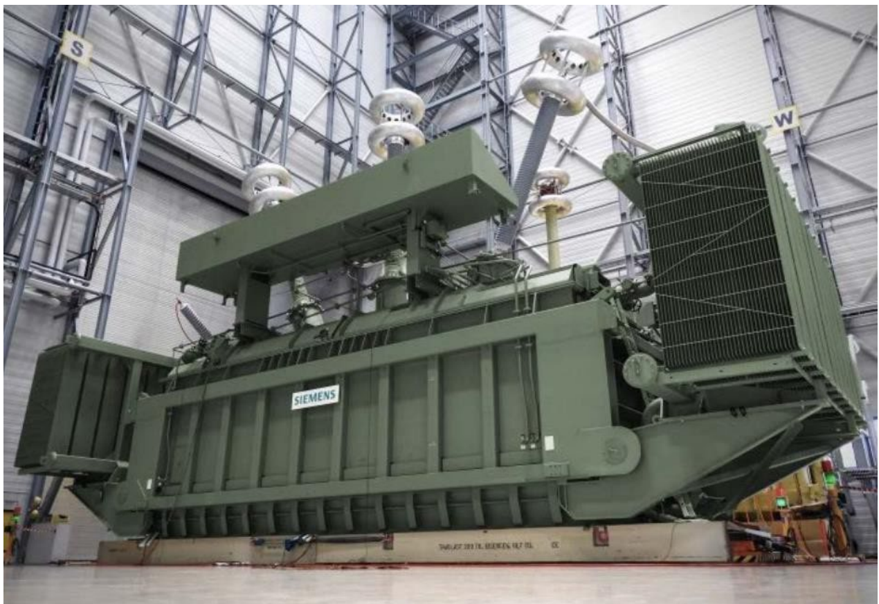
Figure 1-4: Three-phase 420 kV, 50-250 Mvar shunt reactor (length 18.7 m, tank width 4 m, width 7.6 m, tank height 4.5 m, height 11.1 m, transport weight 219,000 kg, operating weight 361,000 kg). Source [1.1]
