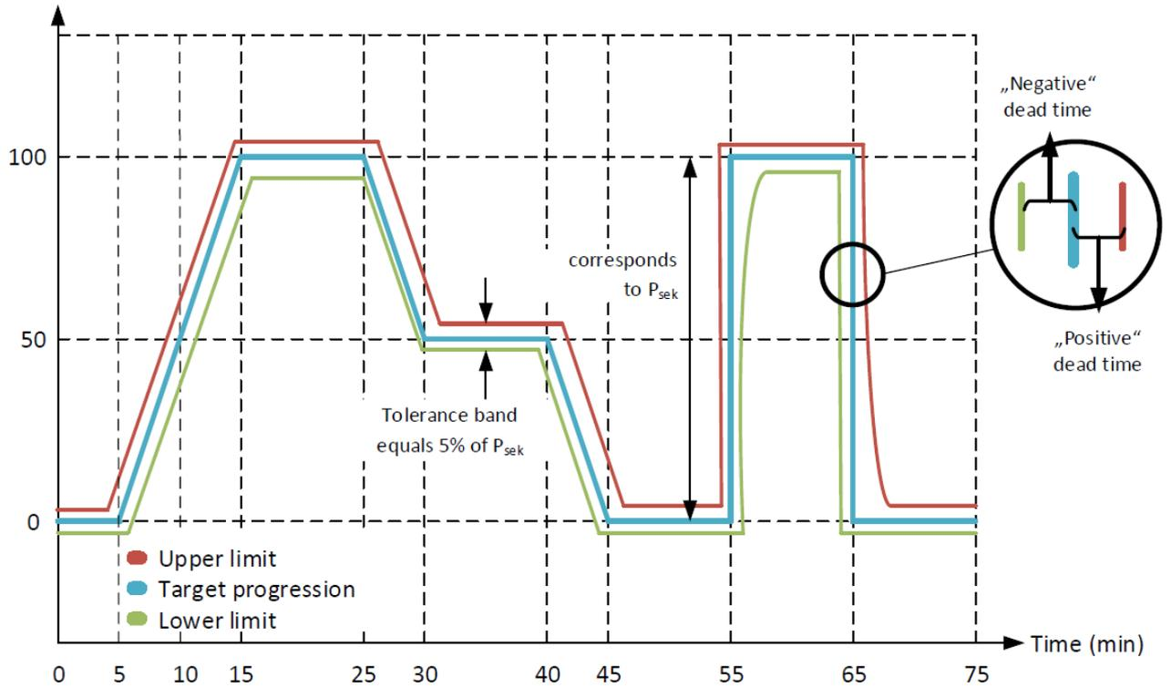
Figure 3: Test signal with tolerance bands for positive secondary control power
