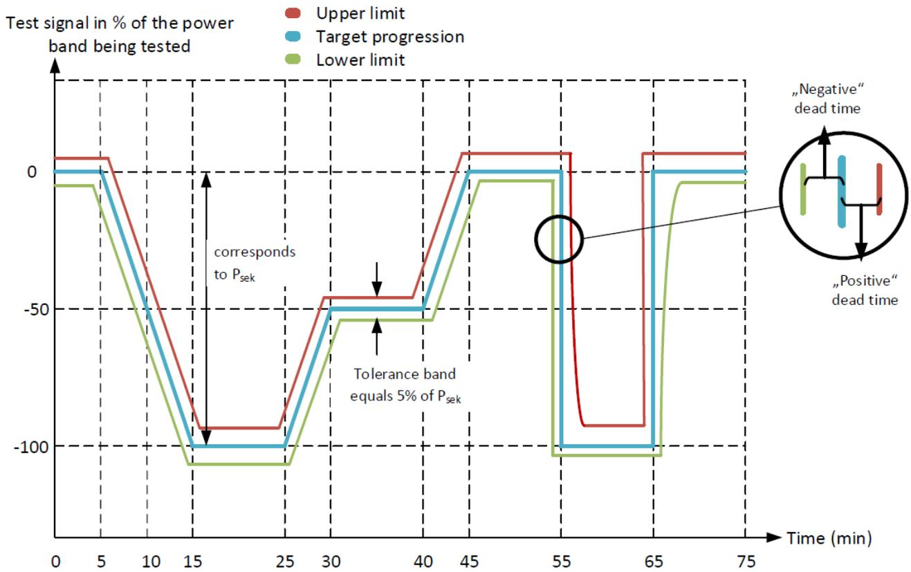
Figure 2 1: Test signal with tolerance bands for secondary control power
