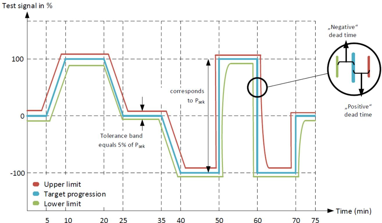
Figure 1: Test signal with tolerance bands
